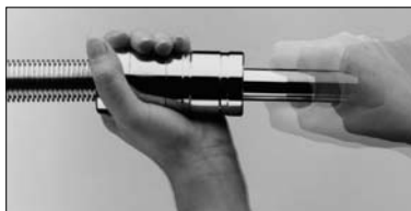
4. Close clamping jaws. Move the striking pin to compress the corrugation into a flange.
