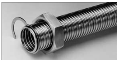
6. Insert clamp ring in the first corrugation groove and press together to form a closed ring. Insert seal, position threaded insert and use two spanners to tighten.
