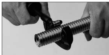
1. Cut hose to required length in the corrugation groove using a pipe cutter.
