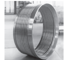
Fig. 8.6 Axial expansion joint made of Alloy 825 for heat exchanger (DN 1200/PN 40)
