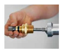
3. Insert the pull rod into the HYDRA GS axial pressing tool, with the mounted fitting.
